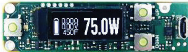
Printed circuit board with a chipset and display screen for a box mod
